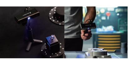
Effortlessly get scans using the MINI as a handheld or fixed scanner with a motorized turntable. Scan a wide variety of objects for all kinds of 3D modeling needs using either the MINI's marker or feature alignment modes.
